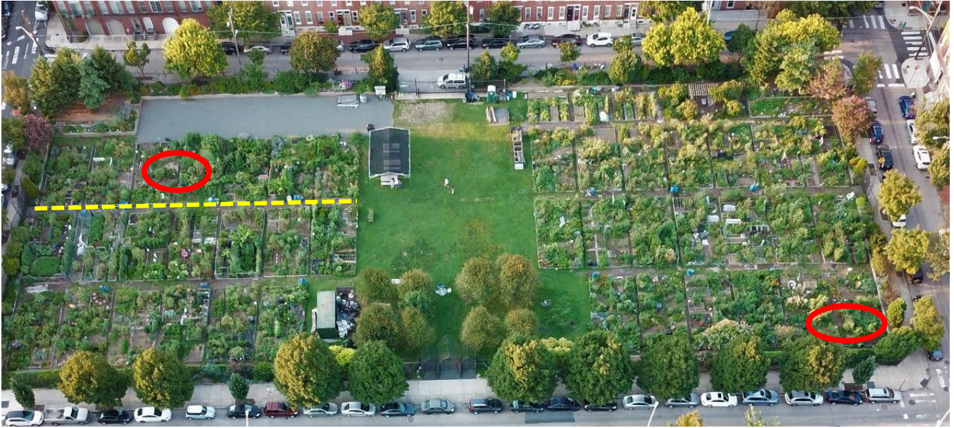
This wonderful aerial view (above) shows the entire 2.6 acre site of The Spring Gardens taken in September 2019. North St. is on top, Wallace St. is below. 19 th St. is to the left, 18 th St is to the right. The yellow dashed line is along the east/west path where the first trench has been dug. The red ovals crudely demarcate areas of TSG that are sinking. Photo by Nick Gruberg.
